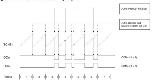
The Timer/Counter Overflow Flag (TOV2) is set each time the counter reaches MAX. If the interrupt is enabled, the interrupt handler routine can be used for updating the compare value.
