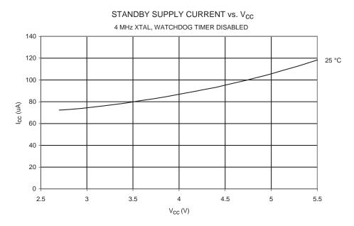
Figure 166. Standby Supply Current vs.  $V_{\text{CC}}$  (4 MHz Resonator, WDT Disabled)
