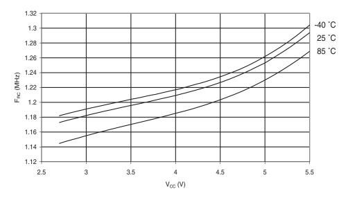
Figure 189. Calibrated 8 MHz RC Oscillator Frequency vs. Temperature
