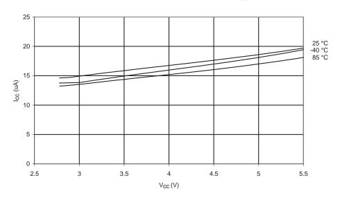
Figure 202. ADC Current vs. V<sub>CC</sub> (AREF = AVCC)
