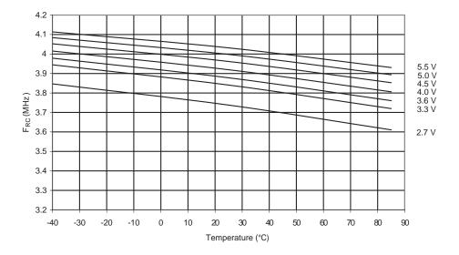
Figure 193. Calibrated 4 MHz RC Oscillator Frequency vs.  $V_{\rm CC}$
