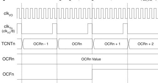
Figure 36. Timer/Counter Timing Diagram, Setting of OCF0, with Prescaler (f<sub>clk\_l/O</sub>/8)
