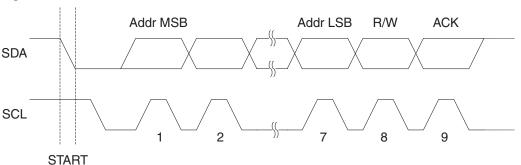
Figure 79. Address Packet Format
