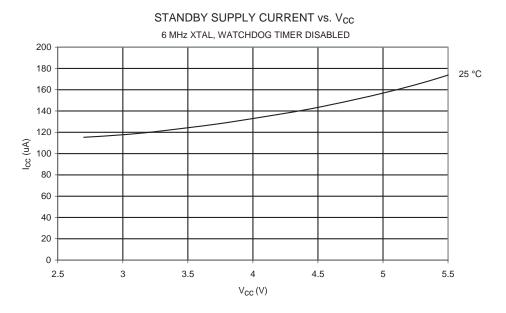
Figure 164. Standby Supply Current vs. V<sub>CC</sub> (6 MHz Resonator, WDT Disabled)
