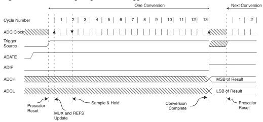
Figure 104. ADC Timing Diagram, Free Running Conversion
