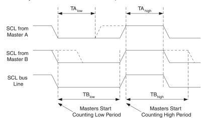
Figure 82. SCL Synchronization between Multiple Masters
