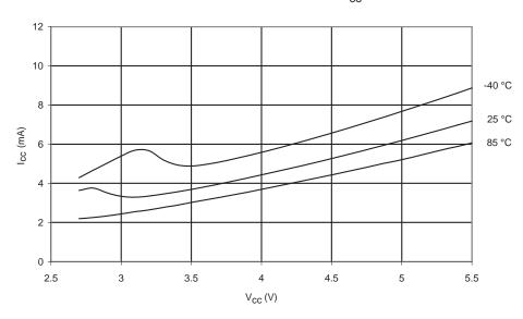
Current Consumption in Reset and Reset Pulsewidth
