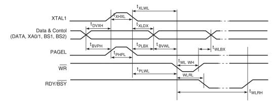
**Figure 134.** Parallel Programming Timing, Loading Sequence with Timing Requirements<sup>(1)</sup>
