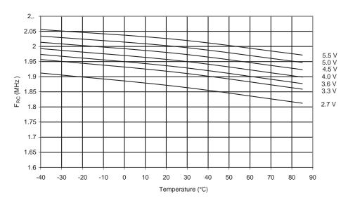
Figure 196. Calibrated 2 MHz RC Oscillator Frequency vs.  $V_{\rm CC}$
