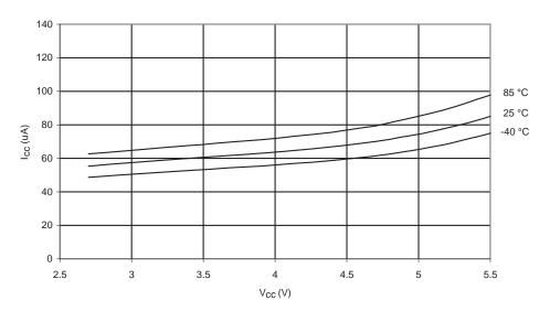
Figure 205. Programming Current vs. V<sub>CC</sub>
