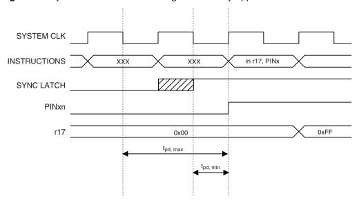
Consider the clock period starting shortly *after* the first falling edge of the system clock. The latch is closed when the clock is low, and goes transparent when the clock is high, as indicated by the shaded region of the "SYNC LATCH" signal. The signal value is latched when the system clock goes low. It is clocked into the PINxn Register at the
