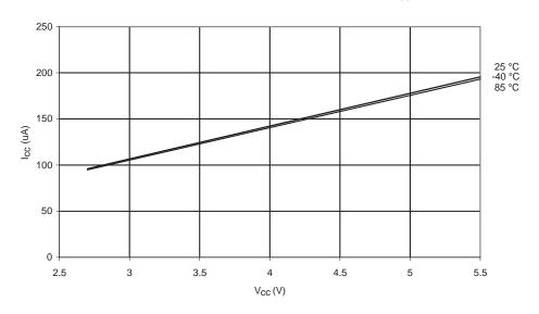
Figure 204. Analog Comparator Current vs. V<sub>CC</sub>
