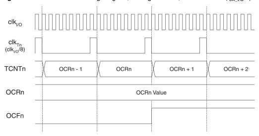
Figure 63 shows the setting of OCF2 and the clearing of TCNT2 in CTC mode.
