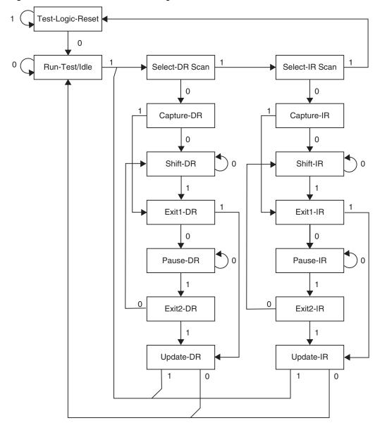
Figure 113. TAP Controller State Diagram
