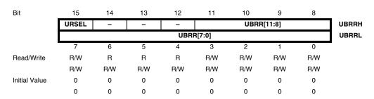
The UBRRH Register shares the same I/O location as the UCSRC Register. See the "Accessing UBRRH/ UCSRC Registers" on page 158 section which describes how to access this register.
