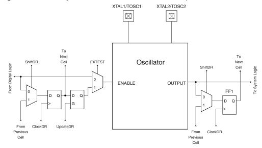
Table 89 summaries the scan registers for the external clock pin XTAL1, Oscillators with XTAL1/XTAL2 connections as well as 32 kHz Timer Oscillator.
