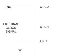
When this clock source is selected, start-up times are determined by the SUT fuses as shown in Table 12.
