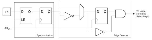
The synchronization and edge detector logic introduces a delay of 2.5 to 3.5 system clock cycles from an edge has been applied to the T1/T0 pin to the counter is updated.
