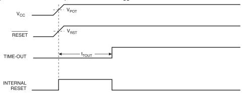
Figure 17. MCU Start-up, RESET Extended Externally
