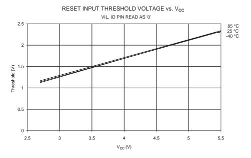
Figure 184. Reset Input Pin Hysteresis vs.  $V_{\rm CC}$
