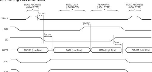
**Figure 135.** Parallel Programming Timing, Reading Sequence (within the Same Page) with Timing Requirements<sup>(1)</sup>
