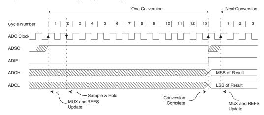
Figure 103. ADC Timing Diagram, Auto Triggered Conversion
