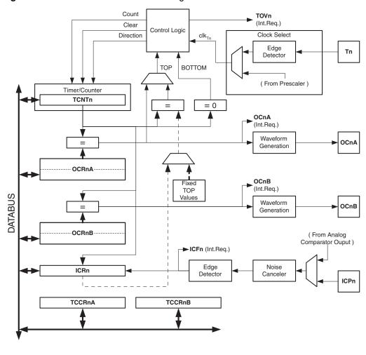
Figure 40. 16-bit Timer/Counter Block Diagram<sup>(1)</sup>
