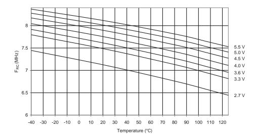
Figure 190. Calibrated 8 MHz RC Oscillator Frequency vs.  $V_{\rm CC}$
