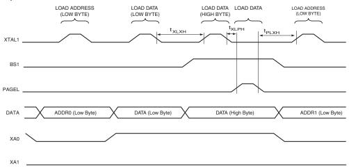
Note: 1. The timing requirements shown in Figure 133 (i.e.,  $t_{DVXH}$ ,  $t_{XHXL}$ , and  $t_{XLDX}$ ) also apply to loading operation.
