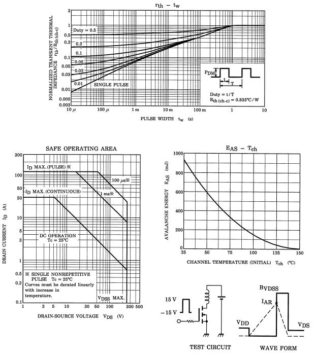
$\begin{array}{ll} \mathrm{R_{G}=25~\Omega} \\ \mathrm{V_{DD}=50~V,~L=1.74~mH} \end{array} & \mathrm{E_{AS}=\frac{1}{2}\cdot L\cdot I^{2}\cdot \left(\frac{\mathrm{B}\mathrm{VDSS}}{\mathrm{B}\mathrm{VDSS}-\mathrm{V}\mathrm{DD}}\right) } \end{array}$
