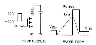
$$\begin{aligned} R_G &= 25~\Omega \\ V_{DD} &= 90~V,~L = 4.3~mH \end{aligned} \qquad E_{AS} &= \frac{1}{2} \cdot L \cdot I^2 \cdot \left( \frac{BVDSS}{BVDSS - V_{DD}} \right) \end{aligned}$$
