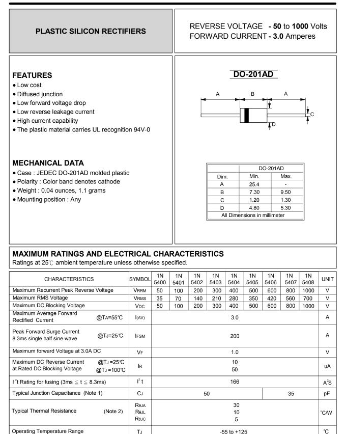
NOTES : 1.Measured at 1.0MHz and applied reverse voltage of 4.0V DC.
