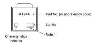
Note 1: A line under a Lot No. identifies the indication of product Labels. Not underlined: [[Pb]]/INCLUDES > MCV Underlined: [[G]]/RoHS COMPATIBLE or [[G]]/RoHS [[Pb]]
