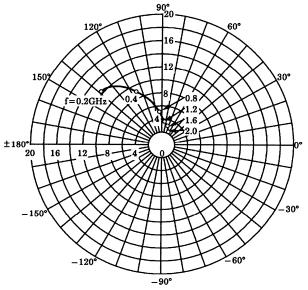
$\begin{array}{c} S_{12e} \\ V_{CE} = 6V \\ I_{C} = 3mA \\ Ta = 25^{\circ}C \end{array}$
