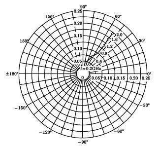
$\begin{array}{l} \text{S}_{22e} \\ \text{V}_{\text{CE}} = 6\text{V} \\ \text{I}_{\text{C}} = 3\text{mA} \\ \text{Ta} = 25^{\circ}\text{C} \\ \text{(UNIT}: \Omega) \end{array}$ j50 j25 j100 j150 j10 10 250 f=0.2GHz
