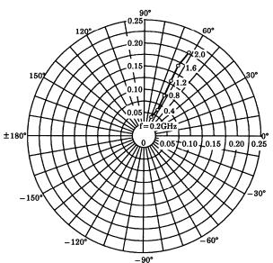
$S_{22e}$   $V_{CE} = 6V$   $I_{C} = 7mA$   $T_{a} = 25^{\circ}C$  (UNIT : O)
