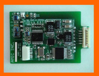
AMIC's A9262-A-000 reader module is a high performance and small formfactor 13.56MHz contactless reader system with integrated antenna. It is designed specifically for embedded application where automated tag ID detection is required.
