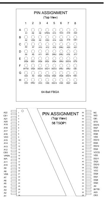
ASI's, AS28F128J3M Enhanced or Mil-Temp variant of Micron's This device features in-system block locking. They also have a Common FLASH Interface [CFI] that permits software algorithms to be used for entire families of devices. The software is deviceindependent, JEDEC ID-independent with forward and backward compatibility.
