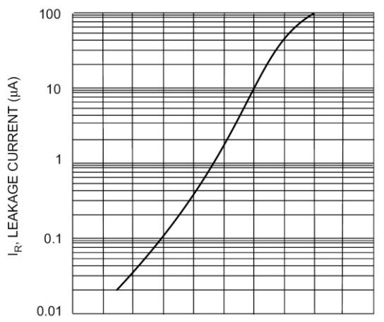
Fig. 3 Leakage Current vs Junction Temperature
