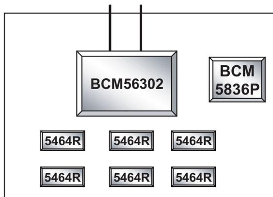
The BCM56302 is the fifth generation of the highly-integrated and cost-effective Broadcom StrataSwitch and StrataXGS product line in a single-chip solution, with 24 GbE ports and two 10-GbE/HiGig+ uplink ports. The BCM56302 is a member of the Value GbE product line, with a corresponding pin-compatible member in the Feature GbE product line—BCM56502. The BCM56302 incorporates 24 GbE ports that can operate 10/100/1000 Mbps. The uplink ports can operate in two modes:
