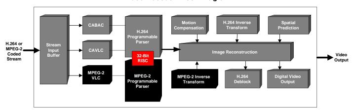
The BCM7411 introduces the advantages of the H.264 video compression algorithm to today's advanced consumer and broadcast applications. The BCM7411 is a dual-channel AVC/MPEG-2 decoder chip capable of full HD real-time decoding.
