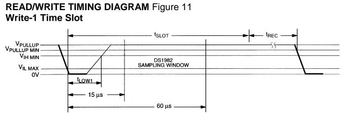
$\begin{array}{l} 60 \ \mu s \leq t_{SLOT} < 120 \ \mu s \\ 1 \ \mu s \leq t_{LOW1} < 15 \ \mu s \\ 1 \ \mu s \leq t_{REC} < \infty \end{array}$
