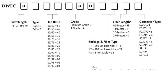
\* The tolerance of fiber length is +/-0.1m. 1 meter is standard. The lead time for special fiber length will be longer.
