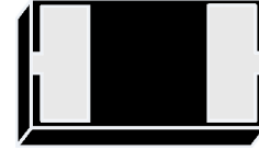
DFN1006-2L (Bottom View)
