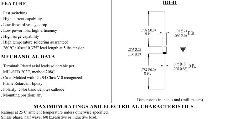
For capacitive load, derate current by 20%
