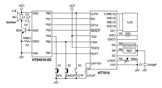
Notes: HT7510's substrate connected to VDD and HT84018-0D's substrate connected to VSS.
