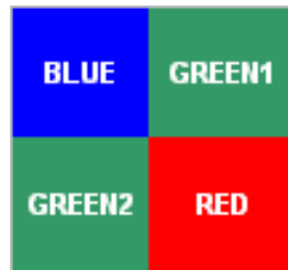
Figure 5: Color filter arrangement on the pixels. Green1 and green2 are separately processed color filters and have a different spectral response. Green1 pixels are located on a blue-green row, green2 pixels are located on a green-red row.
