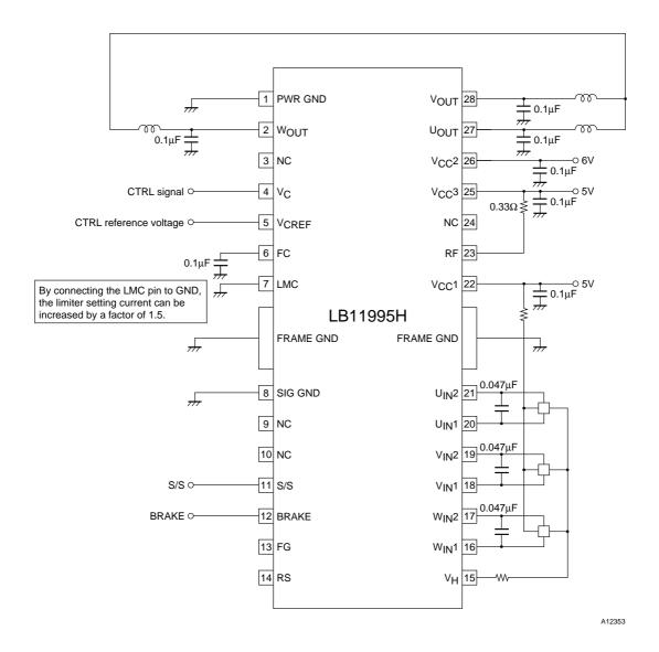
Power supply - GND Output - GND Between Hall inputs Capacitor requirements may change depending on motor. For some motors, capacitor between Hall inputs may not be needed.
