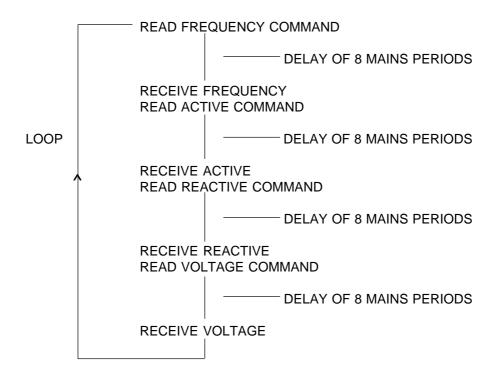
The SA9103C integrated circuit transmits the register values only after completion of the current measurement cycle (8 mains periods maximum).
