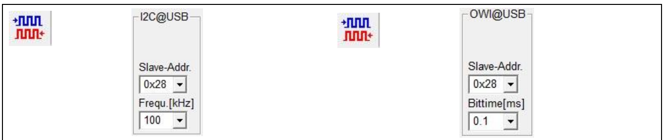
Figure 3.3 Additional I 2 C™ and OWI Interface Settings in the “Send Command” Menu
