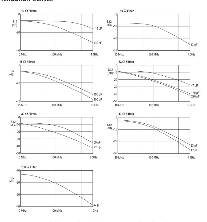
S parameters are measured using a Hewlett Packard HP8753C Network Analyzer with a HP85047A S-parameter Test Set.
