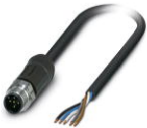
Sensor/actuator cable, 5-position, PE-X halogen-free, black-gray RAL 7021, Plug straight M12, A-coded, on free cable end, cable length: 10 m, for outdoor applications, with high-grade steel knurl
