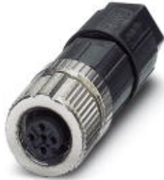
Sensor/actuator connector, socket, straight, 5-pos., M12 SPEEDCON, A-coded, spring-cage connection, metal knurl, cable diameter max. 8 mm
