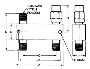
NOTE: All dimensions are  $\pm$  .020, except mounting hole diameters ( $\pm$  .005) and mounting hole location ( $\pm$  .010).
