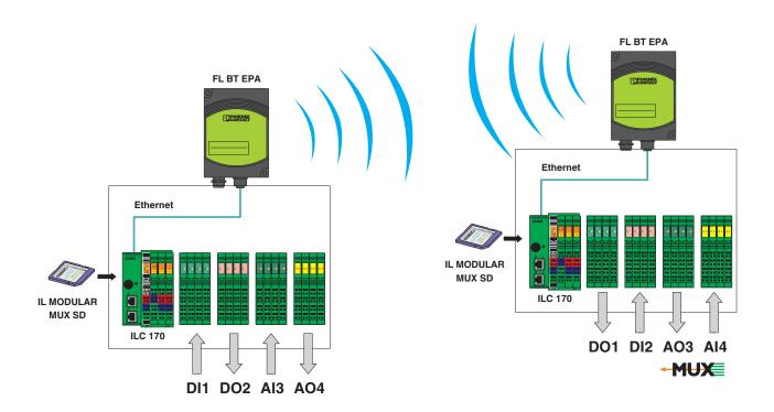
The software on the SD FLASH 512MB MODULAR MUX CompactFlash® card transforms the ILC 131 ETH and the individual input and output terminals required into a flexible field multiplexer. As a wireless connection or as a point-to-point connection in an Ethernet network.
