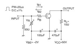
I<sub>C</sub>=10I<sub>B1</sub>= -10I<sub>B2</sub>=5A For PNP, the polarity is reversed.
