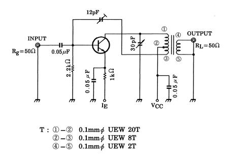
Figure 1 NF, Gpe Test Circuit
