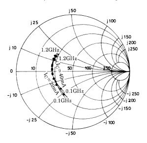
S21e :  $V_{CE} = 10V$ f = 100MHz, 200 to 1200MHz (200MHz step)
