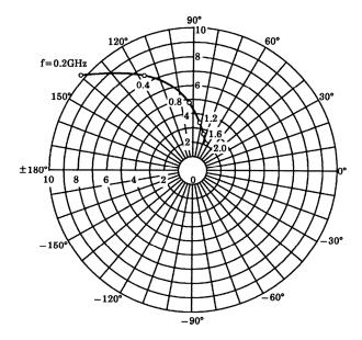
$S_{12e}$   $V_{CE} = 5V$   $I_{C} = 5mA$   $T_{a} = 25^{\circ}C$
