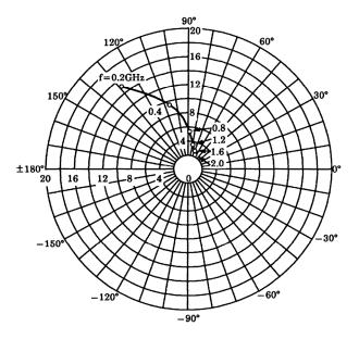
$\begin{array}{l} S_{12e} \\ V_{CE} = 5V \\ I_{C} = 10 mA \\ Ta = 25 ^{\circ}C \end{array}$
