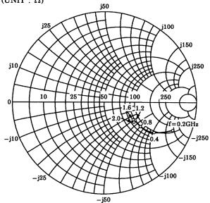
$\begin{array}{l} S_{11e} \\ V_{CE} = 5V \\ I_{C} = 10 mA \\ Ta = 25 ^{\circ}C \\ (UNIT: \Omega) \end{array}$
