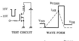
$\begin{array}{ll} R_{G} = 25\Omega \\ V_{DD} = -50V, \ L = 12.6mH \end{array} \quad E_{AS} = \frac{1}{2} \cdot L \cdot I^{2} \cdot (\frac{B_{VDSS}}{B_{VDSS} - V_{DD}}) \end{array}$
