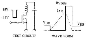
$R_G = 25\Omega$  $E_{AS} = \frac{1}{2} \cdot L \cdot I^{2} \cdot (\frac{B_{VDSS}}{B_{VDSS} - V_{DD}})$ BVDSS  $V_{DD} = -50V, L = 12.6mH$
