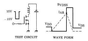
$$\begin{array}{ll} R_G\!=\!25\Omega \\ V_{DD}\!=\!-25V,\; L\!=\!14.84mH \end{array} \quad E_{AS}\!=\!\frac{1}{2}\cdot L\cdot I^2\cdot (\frac{B_{VDSS}}{B_{VDSS}\!-\!V_{DD}}) \end{array}$$
