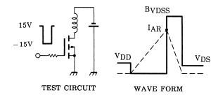
$$\begin{array}{ll} R_G \!=\! 25\Omega \\ V_{DD} \!=\! -50V, \; L \!=\! 10.5 \text{mH} \end{array} \quad E_{AS} \!=\! \frac{1}{2} \cdot L \cdot I^2 \cdot (\frac{B_{VDSS}}{B_{VDSS} \!-\! V_{DD}})$$
