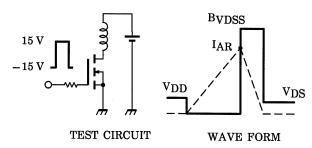
$$\begin{aligned} &R_G = 25~\Omega \\ &V_{DD} = 50~V,~L = 4.2~mH \end{aligned} \qquad EAS = \frac{1}{2} \cdot L \cdot I^2 \cdot \left( \frac{BVDSS}{BVDSS - VDD} \right)$$
