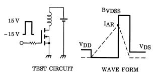
$$\begin{aligned} R_G &= 25~\Omega \\ V_{DD} &= 90~V,~L = 7.35~mH \end{aligned} \quad E_{AS} &= \frac{1}{2} \cdot L \cdot I^2 \cdot \left( \frac{B_{VDSS}}{B_{VDSS} - V_{DD}} \right) \end{aligned}$$
