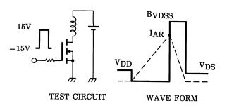
$$\begin{aligned} &RG = 25~\Omega \\ &V_{DD} = 90~V,~L = 43.6~mH \end{aligned} \qquad EAS = \frac{1}{2} \cdot L \cdot I^2 \cdot \left( \frac{BVDSS}{BVDSS - VDD} \right) \end{aligned}$$
