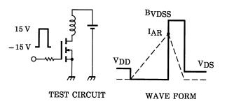
$$\begin{aligned} &R_G = 25~\Omega \\ &V_{DD} = 50~V,~L = 1.74~mH \end{aligned} \qquad E_{AS} = \frac{1}{2} \cdot L \cdot I^2 \cdot \left( \frac{BVDSS}{BVDSS - V_{DD}} \right) \end{aligned}$$
