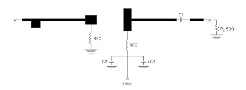
= Microstrip on 0.020" Teflon Fiberglass, Er=2.55 C1,C2 = ATC 'A' 47pf C3 =  $10\mu fd$  @ 35 Volts
