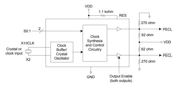
Output resistors shown are for unterminated lines. Refer to MAN09 for additional information.
