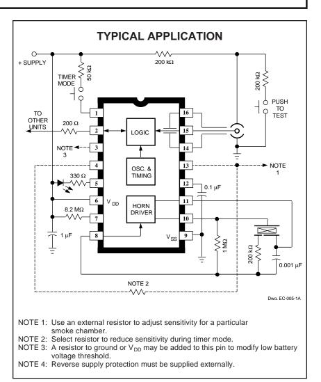
sound their associated horns after a nominal 3 second delay. The LED remains ON when an alarm is signaled from an interconnected unit and a local smoke condition does not exist.
