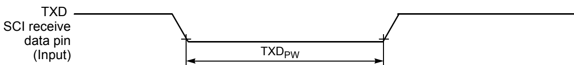
Figure 4-32 TXD Pulse Width
