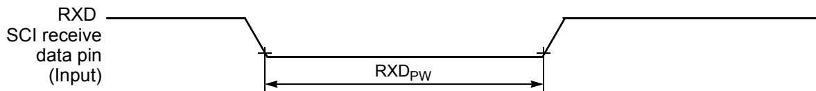
Figure 10-12 RXD Pulse Width
