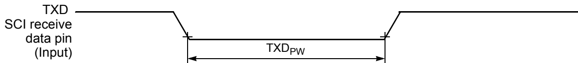
Figure 10-13 TXD Pulse Width
