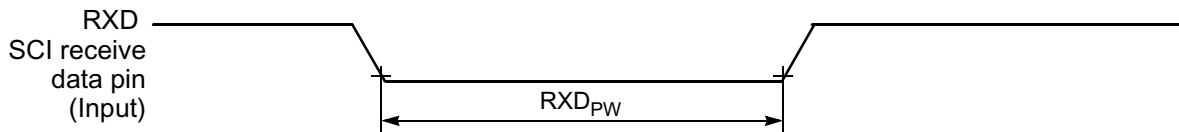
Figure 10-15 RXD Pulse Width
