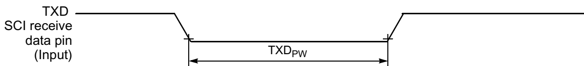
Figure 10-16 TXD Pulse Width
