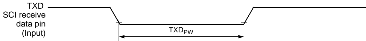
Figure 10-17 TXD Pulse Width
