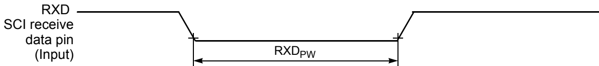
Figure 10-15 RXD Pulse Width
