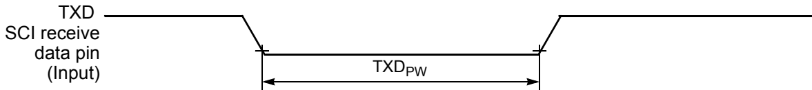
Figure 10-16 TXD Pulse Width
