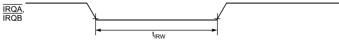
Figure 10-6 External Interrupt Timing (Negative-Edge Sensitive)
