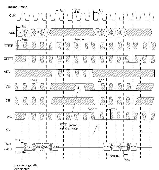
$\overline{\text{WE}}$  is the combination of  $\overline{\text{BWE}}$ ,  $\overline{\text{BW}}_{[1:0]}$ , and  $\overline{\text{GW}}$  to define a write cycle (see Write Cycle Descriptions table).  $\overline{\text{CE}}$  is the combination of  $\overline{\text{CE}}_2$  and  $\overline{\text{CE}}_3$ . All chip selects need to be active in order to select the device. RAx stands for Read Address X, WAx stands for Write Address X, Dx stands for Data-in X, Qx stands for Data-out X.
