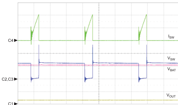
Figure 3. Expanded view of Timer mode: V_{OUT} \leq 10 V, V_{BAT} = 5.5 V, Ch1: V_{OUT} = 20 V/div., Ch2: V_{BAT} = 5 V/div., Ch3: V_{SW} = 5 V/div., Ch4: I_{SW} = 500 mA/div., t = 5 \mu s/div.
