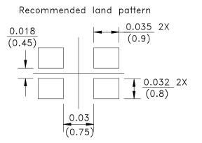
**Note:** From the top view (marking side), pin #1 is always located at the bottom left corner of the package. This is regardless of the location of the Chamfer, since due to material availability, the Chamfer could be located on pin#1, 2 or 4. Be advised that the Chamfer location has no impact on the electrical performance of the device.
