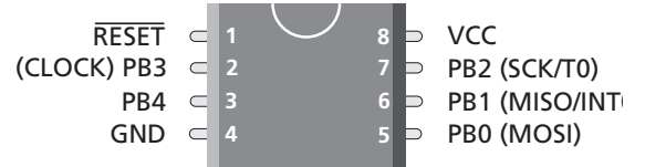
Pinout for the AT90S2343
